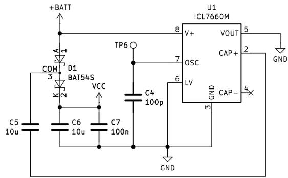
The expected current load of the charge pump is lower than 1 mA. For this light load, we will lower the oscillation frequency to 1 kHz to increase efficiency. The output source resistance will be  $\pm 100 \Omega$  for temperatures between  $-25^\circ\text{C}$  and  $50^\circ\text{C}$  and supply voltages in the range of 1.5–2.8 V.
